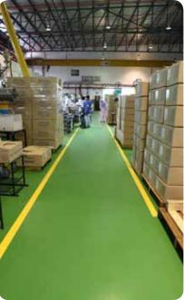
Surface unevenness can lead to excessive vibration on a lift truck and increase down time and repairs. Exact floor flatness is crucial to ensure operations are more effective if lift trucks can operate at maximum speed. With flat floors, Health & Safety is increased while operator tiredness is decreased. The risk of damage to stock is also decreased with no risk of racking collapsing as a result of uneven surfaces.
